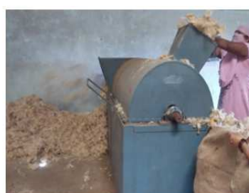
Figure 4: Opening and Dusting of UAS Sheep Breed Wool
