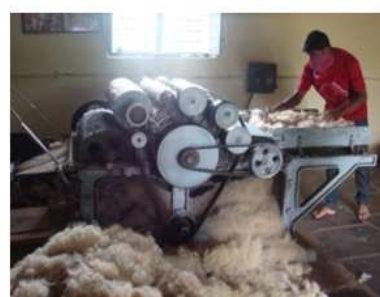
Figure 6: Pre-Carding of UAS Wool Fibres
