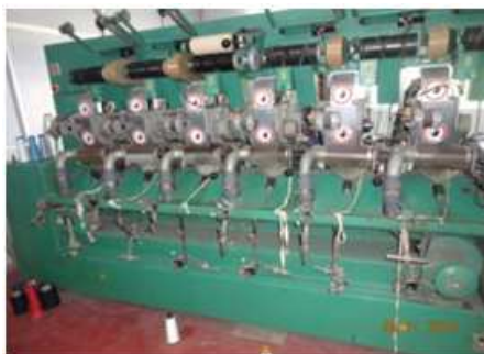
Figure 9: Friction Spinning of UAS Sheep Breed Wool Blended Yarns
